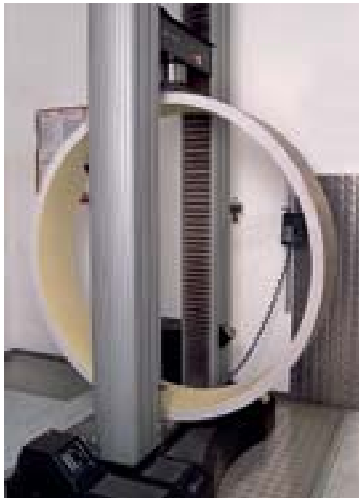
Fig. 44: Ring deflection test
