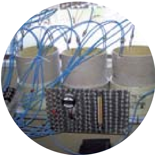
Fig. 29: Test configuration – long-term sealing pressure
