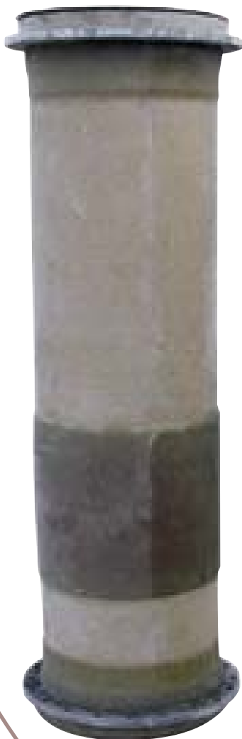
Biaxially loaded pipe with laminate
