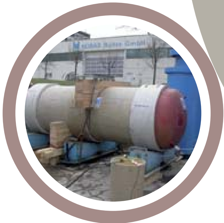
Fig. 24: Test for misalignment by shear load and draw on HOBAS® locked joint system DN 1200 PN 6
