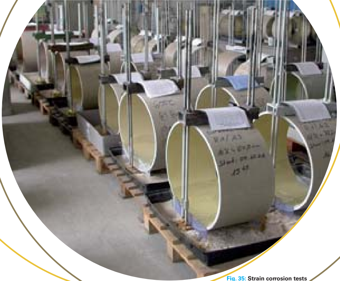
Fig. 35: Strain corrosion tests
